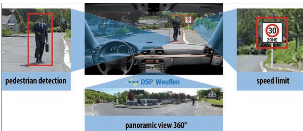
Fig. 5. Full-digital 360° round-view driver assistance system with active pedestrian detection. (picture: DSP-Weuffen)
